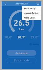
3 Device Setting Interface In this interface, you can view device type and device ID, and you can set device tag, device icon and the Anti-Frozen Protection function.
